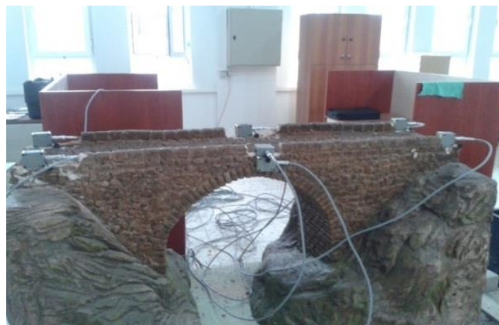
Fig. 2. Test setup of reduced-scaled bridge model.
